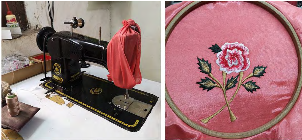
Figure 2. The embroidery sewing machine (left) and embroidery hoop (right).
